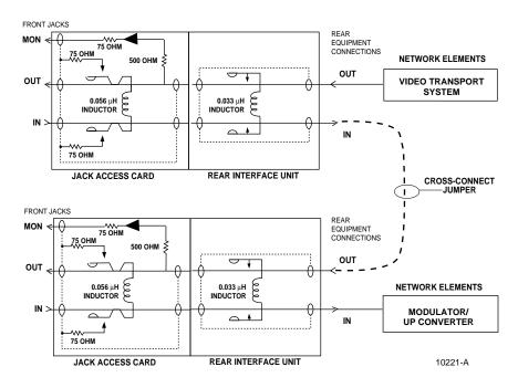
Figure 25. Typical Cross-Connect Application
